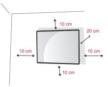
If you want to mount the monitor on the wall (optional), attach the wall mounting bracket to the rear of the monitor.
